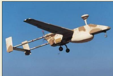
major subsystems on a manned aircraft. The Rustam, a 1.1 ton UAV, is being built to remain aloft for more than 24 hours with a range of up to 300 kilometres and a maximum altitude of 10,000 meters.
