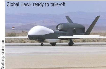
costs about US \$10 million and is powered by an Allison Rolls-Royce AE3007H turbofan engine; it carries a payload of 900 kilograms (2,000 pounds).
